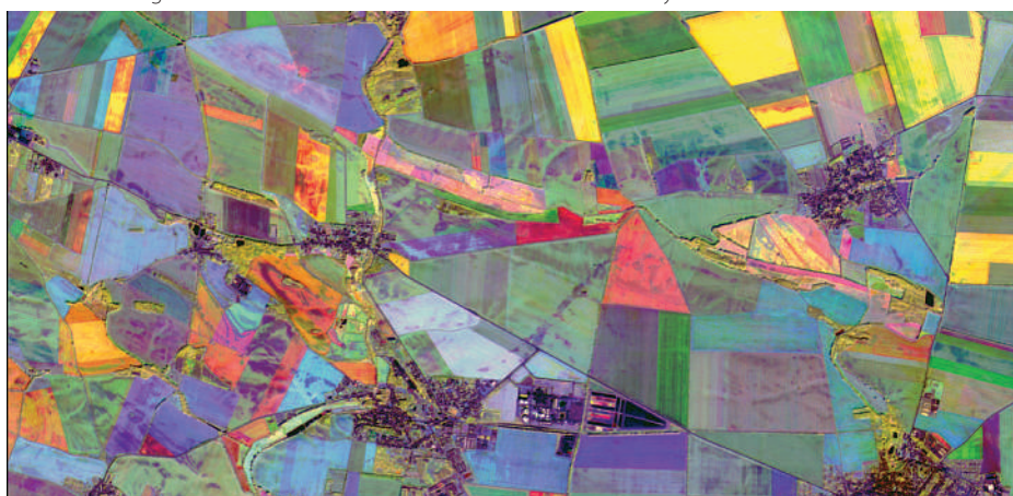
Multi-temporal pseudo-colour image of a rural area in northern Germany. Colours enable the identification of crop types and variability of soil properties and crop vegetation
